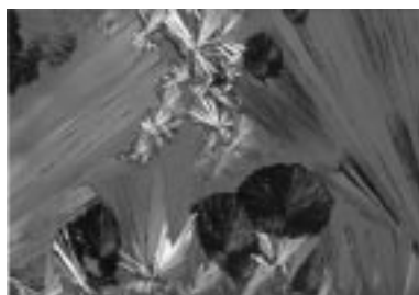
Fig. 13 Propylphenazone. The two enantiotropically related forms may be obtained simultaneously by fast cooling from the melt as observed by thermomicroscopy
